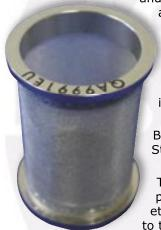
and handling. Weakened baskets will lose their shape and will often fail to comply with the specifications of the USP. Baskets are available in the standard mesh sizes of 10, 20 and 40, with other mesh sizes and PTFE coating available as a custom order.
